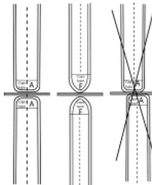
**Caution:** The caps must be perfectly aligned. To check the electrode line, see change of arms on pages 18 and 19.
