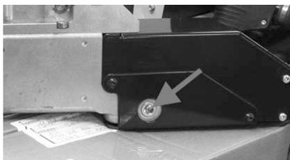
The screw shown opposite ensures secure attachment of the copper cable which carries current to the clamp. It is recommended that screw tightness is checked every month to prevent irreversible damage inside the clamp.
