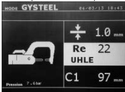
The GYSTEEL mode is identical to normal mode except that the user enters the yield strength of steel. The Ys may be found using a durometer such as Gysteel Vision
