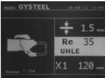
The auto mode is identical to normal mode except that the user enters the yield strength of steel. The Ys may be found using a durometer such as Gypeel Vision
