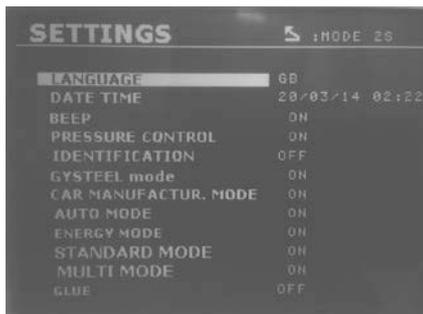
The **SETTINGS** mode can be accessed by pressing the MODE key during more than 2 seconds.
