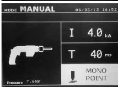
◆ In manual mode, the maximum permitted welding current is 9 kA during a period that will not exceed 600 ms, it is therefore impossible to select higher values for these parameters.
