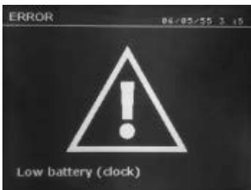
The message « Low battery (clock) » appears after switch ON of the machine and alerts the user that the voltage of the battery on the command board is too low. This battery ensures the saving of the date and time when switching OFF the machine.
