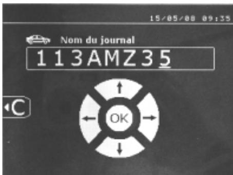
Saving a report allows spot welding data to be stored on a memory card, in order to use it again later or retrieve it at a later date eg. on a computer. GYS supplies software called GYSPOT to read the SD card and the user manual. This GYSPOT software is stored in the SD card with the user manual.
