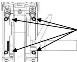
These 4 screws fix the arm to the clamp. They need to be tightened to ensure good transmission of the current. A loose/bad connection leads to loss of current and even worse can cause irreversible damage to the arm or clamp.
