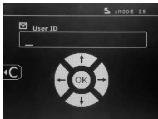
The « left » and « right » arrow keys move the cursor within the field. The up and down arrow keys scroll through letters or figures. Press Esc to erase the field. The Mode button changes the field to modify playback.
