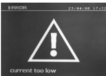
If the welding current measured during the spot is 6% less than the setting, the machine will display the error message “Current too low” - the welding spot should be checked.
