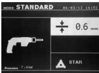
◆ In standard mode, the gun can weld a maximum of 1.5mm thick sheets. When using the gun, the operator can choose between several tools (single spot, carbon shrinking, star welding, studs, rivets, washers, stitches). The tool selection is made with + and - keys.
