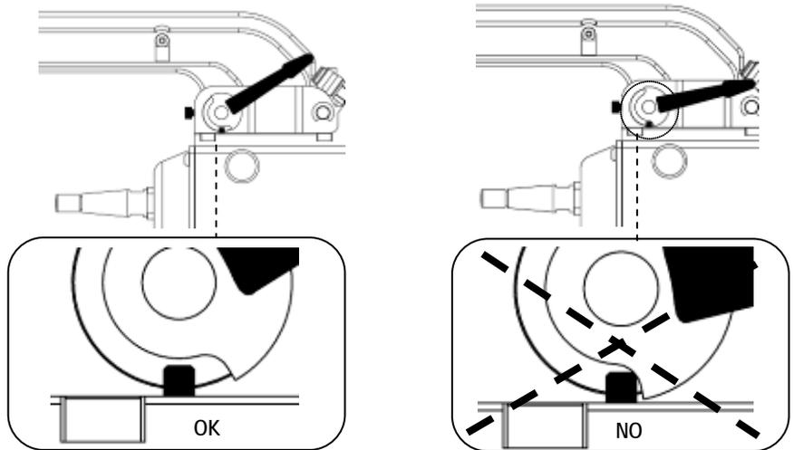
**Warning: Clamp and arm may be damaged if the lever is not tightened properly.**
