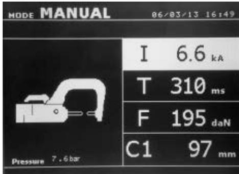
The default settings in manual mode correspond to the settings automatically selected in standard mode (thickness and type of sheet, electrode force, arm). The parameters can be adjusted using the + and – keys (Key Definition diagram, (3) ). The up and down keys allow navigation from one parameter to the next
