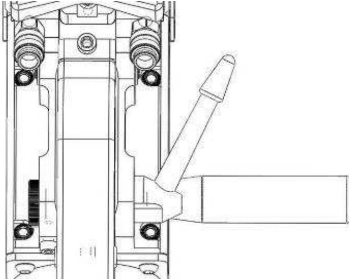
These 4 screws fix the arm to the clamp. They need to be tightened to have a good transmission of the current. A bad tightening leads to a loss of current, and worst can damage your arm or clamp irreversibly.
