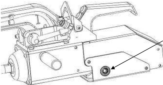
This screw fixes the copper cable terminals to the clamp. The tightening needs to be overhauled or you can have a loss of current or worst you can damage irreversibly your machine.
