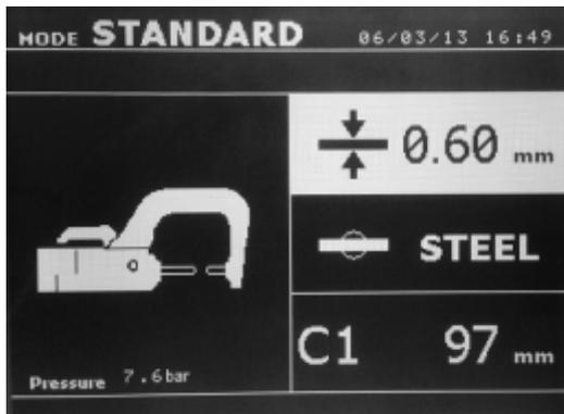
This is the default mode when the machine starts. Quick and easy spot welding by selection of:
