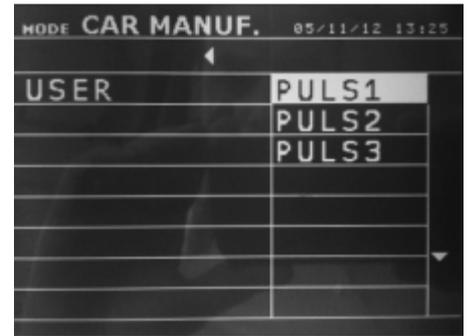
User programmed welding spots can be recalled by selecting USER in the list of car manufacturers. The welding spots can be programmed using the welding spot programming module in the GYSPOT software.
