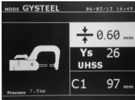
The auto mode is identical to normal mode except that the user enters the yield strength of steel. The Ys may be found using a durometer such as the Gysteel Vision.
