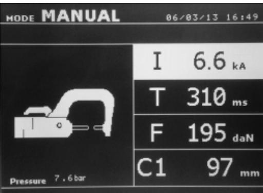
The default settings in manual mode correspond to the settings automatically selected in standard mode (thickness and type of sheet, electrode force, arm).
