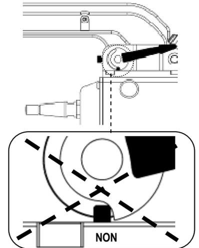
**Warning: Clamp and arm may be damaged if the lever is not tightened properly.**
