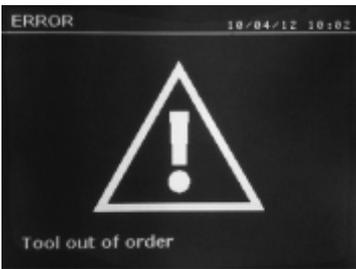
The message « Tool out of order » appears after switch ON of the machine and alerts the user that a button or trigger is constantly pressed, or a permanent short-circuit is detected. Control the trigger of the gun, as well as the buttons on the clamps in order to make this message disappear.
