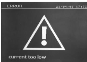
If the welding current measured during the spot is 6% less than the setting, the machine will display the error message "Current too low" - the welding spot should be checked. A message will be displayed at the end of every welding spot, showing the measured welding current. This message is displayed on the screen until a key on the control panel is pressed, or until a new welding spot is performed, by pressing the B button on the clamp.
